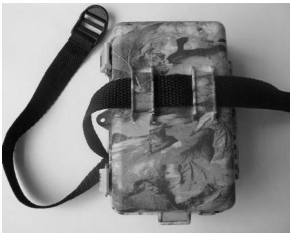
Figure 4: Fixing the camera with belt
